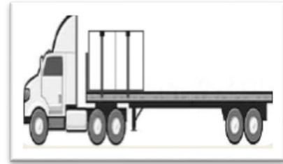
Articles of cargo that are likely to shift, tip or roll must be restrained by chocks, wedges, or a cradle to prevent movement. These restraints must stay fastened or secured while the vehicle is moving.
