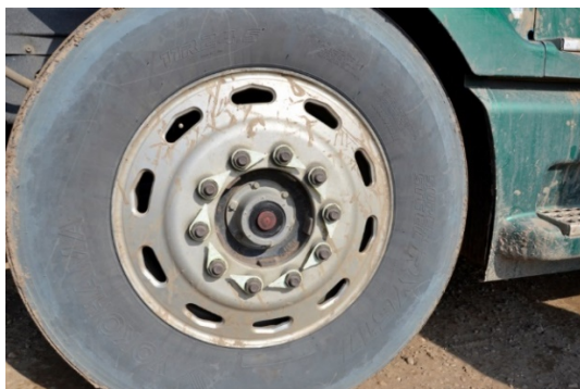
Wheel Fasteners (Nuts, Bolts and Studs)
